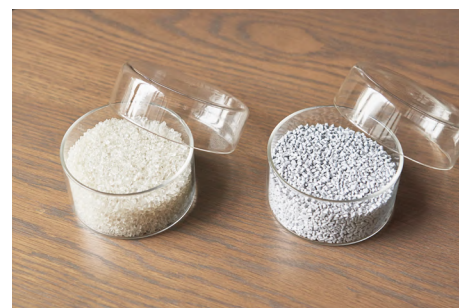
Recycled plastic (right) for the front panel of the product, which uses 80% post-consumer recycled plastic materials (left)
