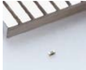
0201 size (0.25mm×0.125mm) ultra-small multilayer ceramic capacitors
