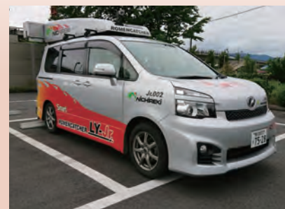
DX compatible road surface condition measuring vehicle SMART ROMEN CATCHER LY Jr.
