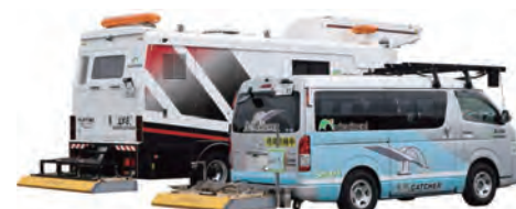
SMART SHOBAN CATCHER (non-destructive bridge deck survey vehicle)
