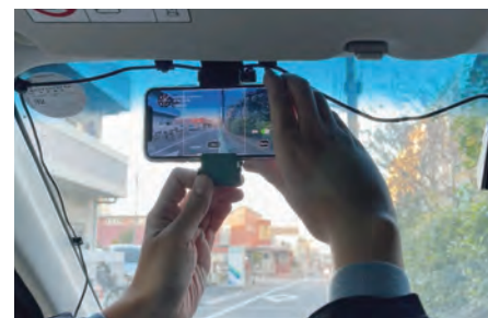
GLOCAL-EYEZ (smartphone-based road inspection system)
