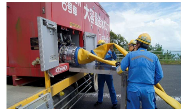
Drill to ensure cooling function using large-capacity pump truck
