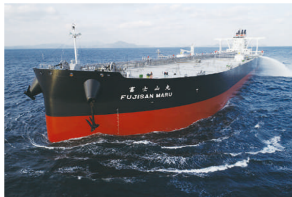
VLCC with SOx scrubber FUJISAN MARU (5th generation)
