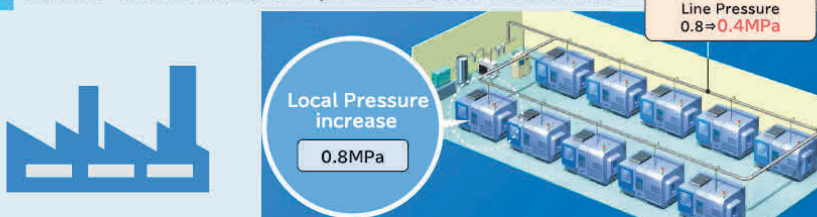
Power saving in factories (reduction of compressor power)
