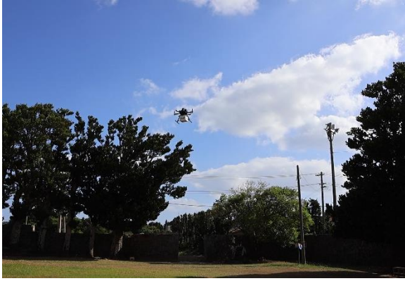
Landing at the delivery destination The cargo is automatically detached and PF2-CAT3 returns to the takeoff point
