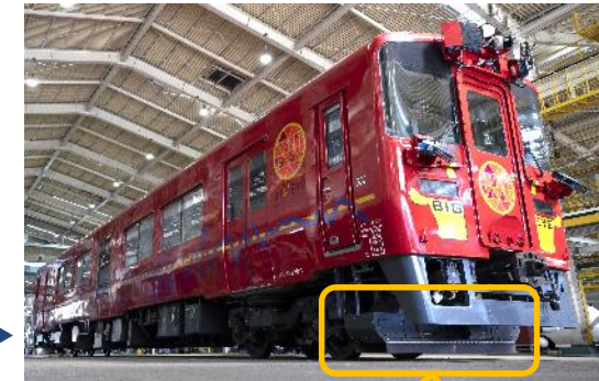
JR Kyushu's multifunctional inspection car "BIG EYE" ▶
