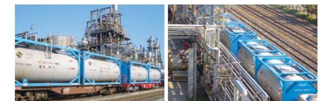
Example of a modal shift: Railway tank containers and loading and refilling facilities
