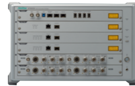
Signaling tester for comprehensive evaluation of wireless terminal applications
