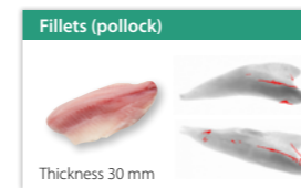
X-ray inspection System. Used to detect contaminants such as metal and stones, and bones that have not been removed.
