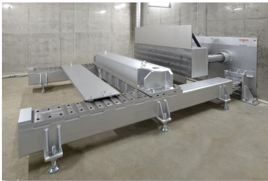
Crush Testing Equipment (No. 1 Safety Test Room)
