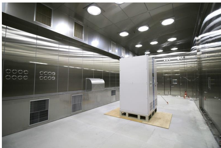
Large Walk-in Type Temperature & Humidity Chamber
