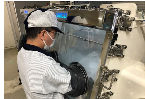
Glovebox for dismantling cells
