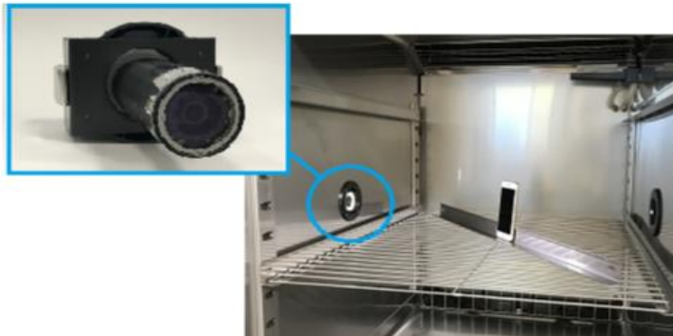
Image of in-chamber monitoring camera
