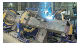
Robotic Welding Systems for Large Pillar Assembly We provide systems to automate welding processes for the steel pillars and beams used in skyscrapers. The use of robotics systems has enabled to strike balance between ensuring welding quality and improving work efficiency.
