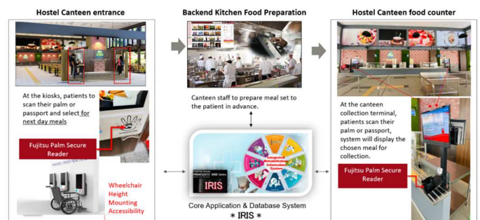
Process of using Fujitsu's palm secure technology to order food in the canteen
