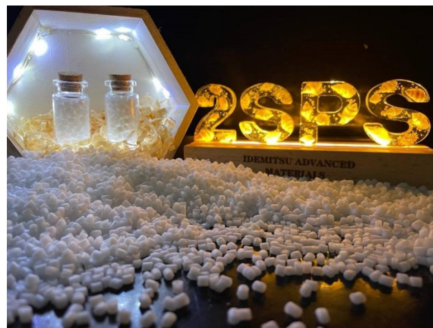
SPS pellet from the 2nd SPS Plant
