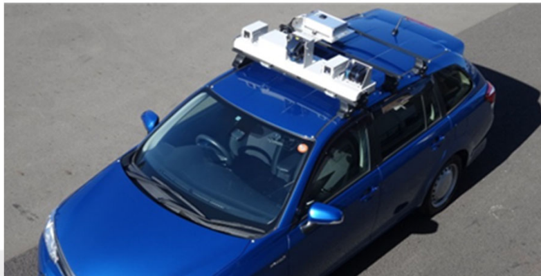
Road Surface Properties Measuring Vehicle
