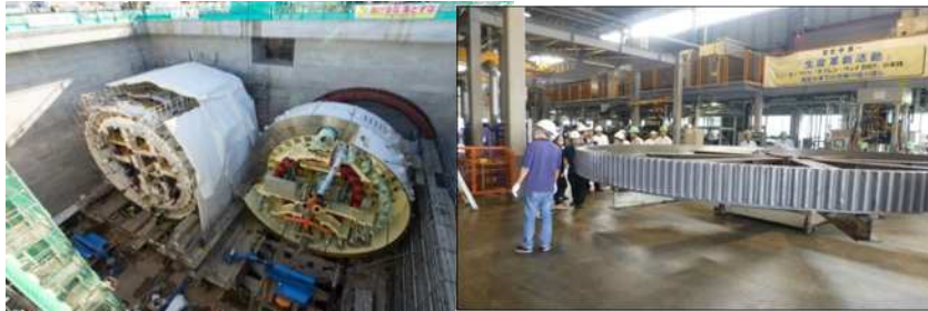
Slewing bearing with gear for tunnel boring machine (outer diameter approx. 8.0m)
