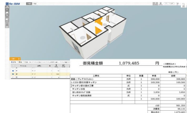
The efficiency of move-out repairs and renovation work will be improved dramatically by utilizing the various information possessed by BIM.
