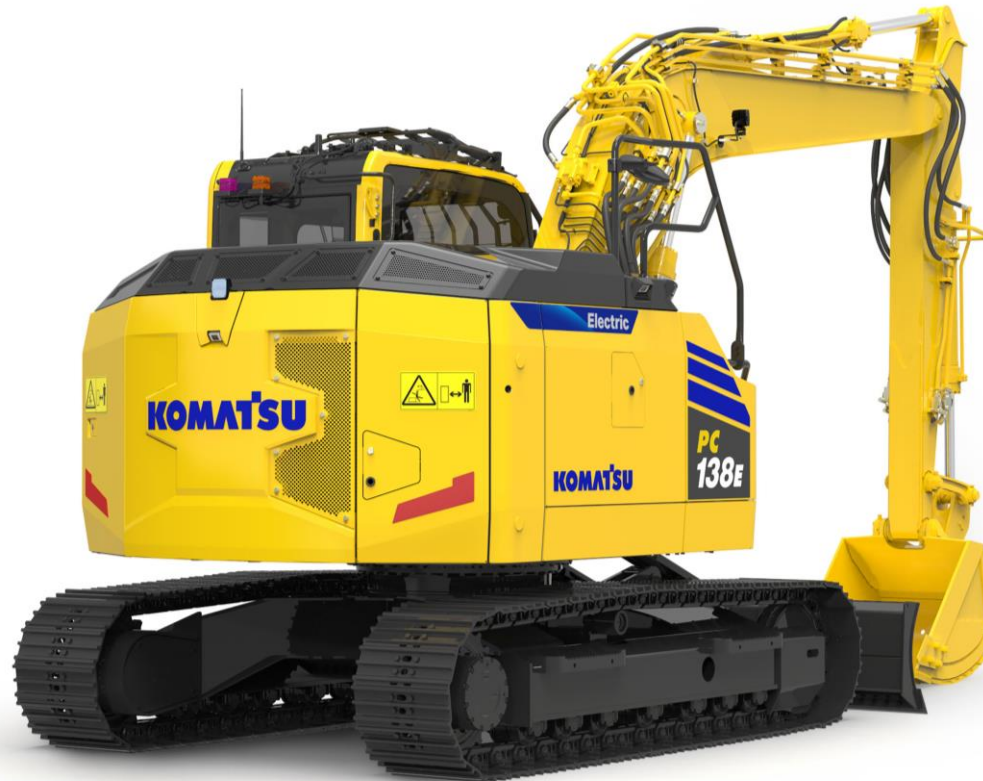
New 13-ton class PC138E-11 electric excavator with a lithium-ion battery
