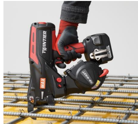
New product of rebar tying tool TWINTIER/increased tying speed
