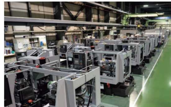
Sliding head stock type automatic lathe production line
