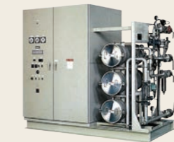
Power supply for ozone generation
