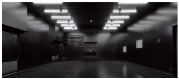
Test chamber: Width 6 m x Depth 9 m x Height 3 m A black coating is applied to suppress the diffuse reflection of light.
