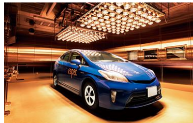
Drive-In Chamber for Vehicle Testing
