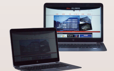
Privacy screen backlight Surface light source to realize privacy mode on the HP Elite Book (2016)
