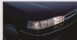
Multi-reflector (MR) headlamp World's first headlamp without ridges in the lens, increasing freedom in car design (1989)
