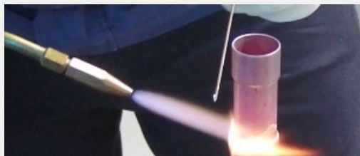
In-house test for using hydrogen in the manufacturing process (Using hydrogen to power brazing burners, etc.)
