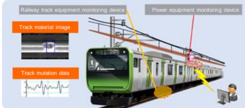
CBM (monitoring of wayside equipment)
